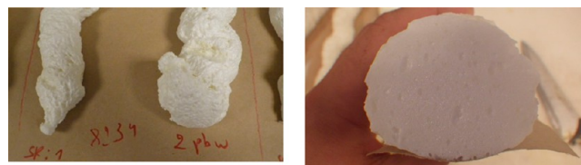
Figure 3. OCF foam 8234 formed with 2 pbw of added CG7 microspheres.
