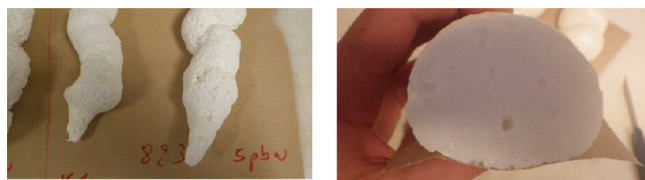
Figure 4. OCF foam 8235 formed with 5 pbw of added CG7 microspheres.
