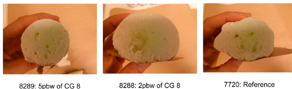
Figure 6. Sections of the OCF foams formed on paper using formulations comprising 2 and 5 pbw of added CG8 microspheres. The 7720 OCF reference foam is also shown.
